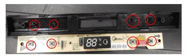
• Install the two Phillip's head screws that secure the board to the housing.
