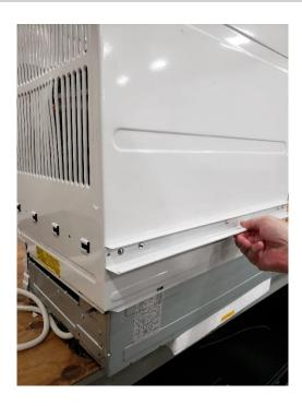
• Install the screws that secure the shell to the unit
