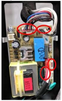
• After all of the electrical connectors are removed, remove the Phillips screw holding the board in the housing
