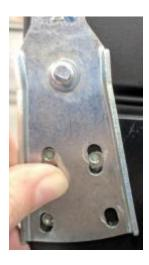
• With a Phillips screwdriver, reinstall the two screws that attach the limiting bracket to the door
