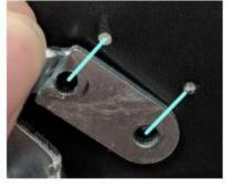
NOTE: The holes for the limiting bracket will be filled with foam. You can simply line the bracket up and screw the screws through the foam
