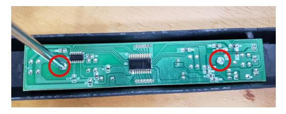
• Slide the new board under the clips and reinstall the two Phillips screws
