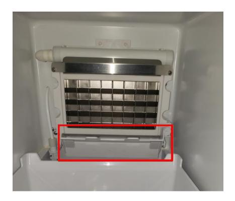
The ice slideway is installed on two pins that pop into wholes on the evaporator bracket.
