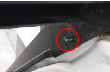
Step 5: Reinstall the lid stopping bar
