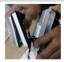
Note— There are some loose parts that may fall out when separating the assembly. These are the holders for the screws and will just need to be lined back up when reassembling the cooling assembly.
