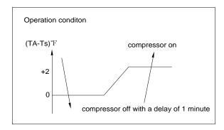
When TA≤TS (for 1 minute) the compressor turns off.
