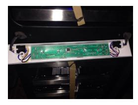
4. Pull out the temperature board and disconnect the wire connector. Replace with new temperature control board.
