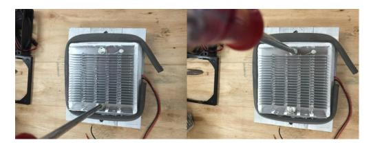
3. Remove the thermoelectric node.
