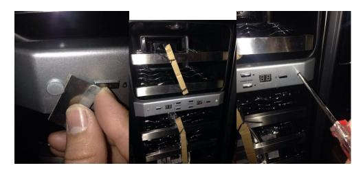
3. Disassemble the temperature control box after removing the screws (2) on the temperature box.
