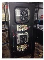
2. Remove the screws (2) on the Thermoelectric Module.
