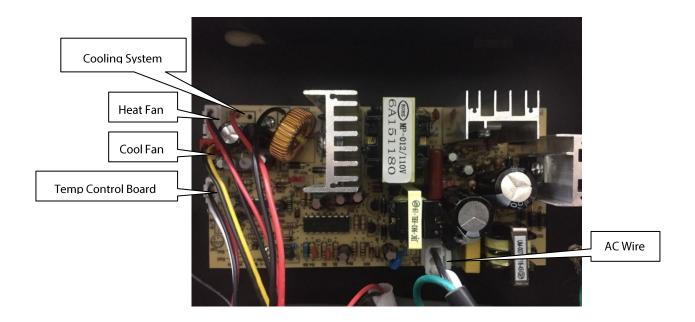
NOTE: All wiring connections need to be attached securely to the board.
