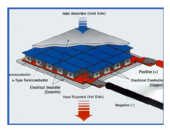
The complete system includes a semi-conductor module (P&N shape semi-conductors clamped with two ceramic chips), an internal and external heat exchanger. To obtain higher energy efficiency low-speed-and-noise fans are fitted to the heat exchangers. During operation direct current goes through the semiconductor module which causes heat to be transferred from one side to the other.
