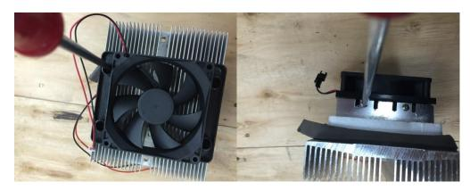
2. Remove screws (2) on the cool sink
