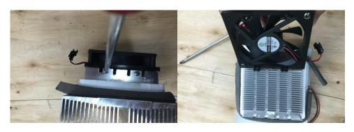
6. When reconnecting the cooling fan make sure to align the bracket in the proper position and reattach the screws (2) to the module.
