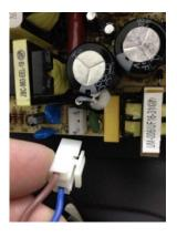
2. Remove screws (4) from the board, desolder the wires (4) from the thermoelectric module.
