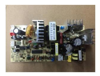
4. Reconnect the connectors on the PCB and resolder the wires from the thermoelectric module.
