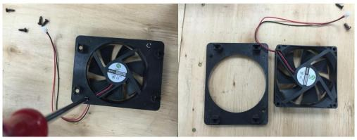
5. When replacing the cooling fan pay attention to the direction of the fan and it's wiring.
