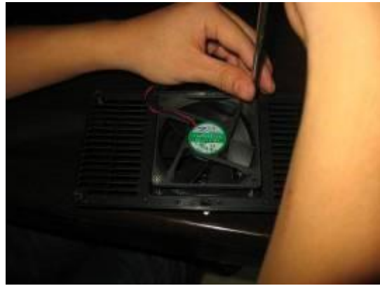
4. Remove the screws (4) from the cooling fan.
