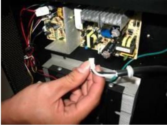
1. Remove the back panel on the unit and disconnect the wire connectors on the board.
