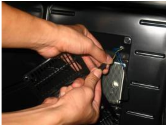
5. Replace the old cooling fan and reconnect the wire.
