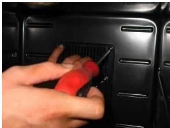
6. Reattach the caps (4) and screws (4).
