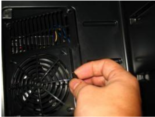
3. Disconnect the wire connector after opening the cooling fan cover.
