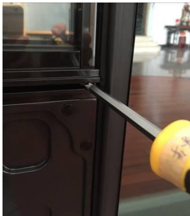
3. Remove screws (2) from the rear of the temperature controller.
