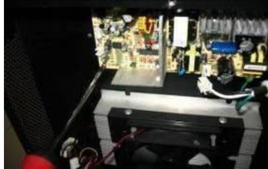
2. Remove screws (4) from the board.
