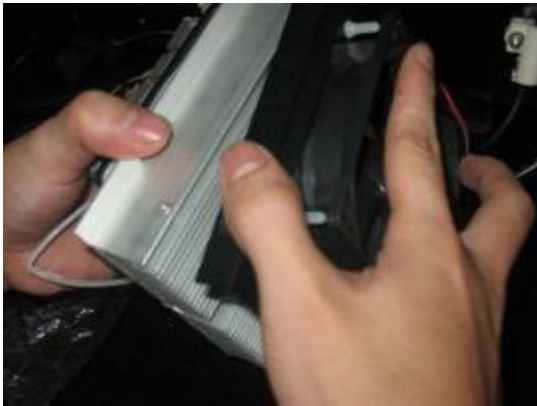
5. Replace the heat fan.
