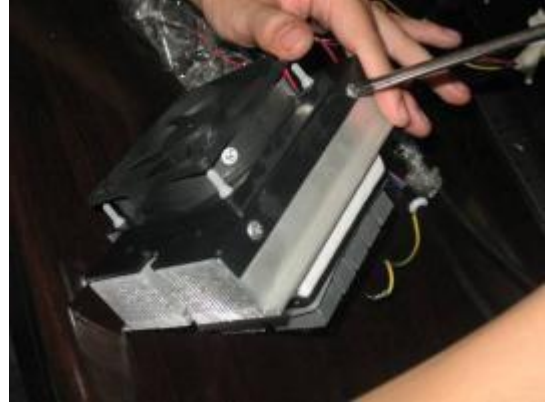
4. Remove the screws (4) from the two sides of heat sink
