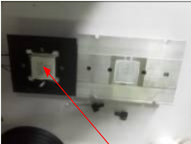
4. Remove old node and apply thermal grease evenly on new node.
