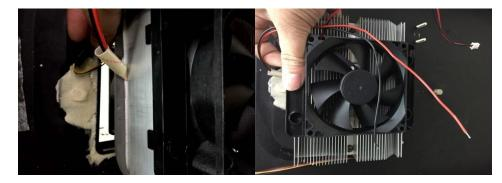
7. Reconnect the wires to the power control board.
