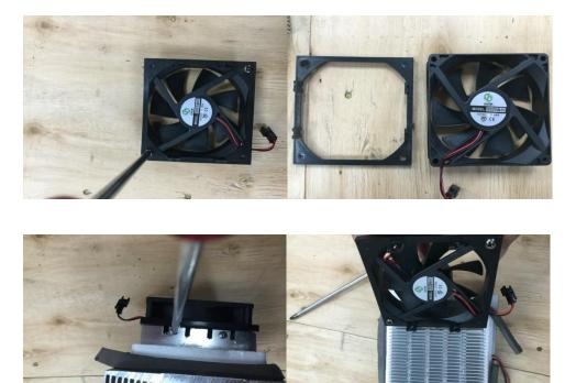
6. When reconnecting the cooling fan make sure to align the bracket in the proper position and reattach the screws (2) to the module.
