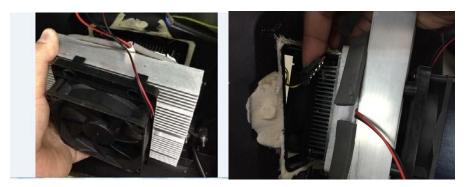
4. When replacing the heating fan pay attention to the direction of the fan and it's wiring.
