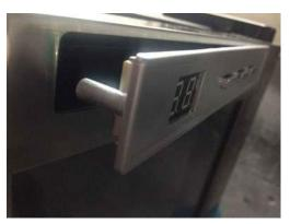
4. Pull out the temperature board and disconnect the wire connector. Replace with a new temperature control board.
