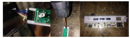
5. Reconnect the wire connector and reassemble the control panel.
