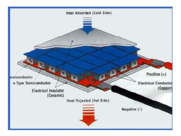
The complete system includes a semi-conductor module (P&N shape semi-conductors clamped with two ceramic chips), an internal and external heat exchanger. To obtain higher energy efficiency low-speed-and-noise fans are fitted to the heat exchangers. During operation direct current goes through the semiconductor module which causes heat to be transferred from one side to the other.
