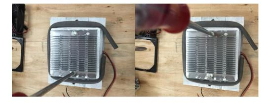
3. Remove the thermoelectric node.
