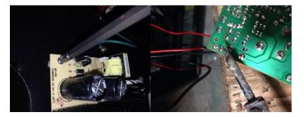
3. Replace the PCB and reattach the screws(4)
