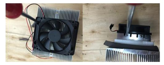
2. Remove screws (2) on the cool sink
