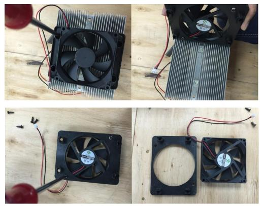
5. When replacing the cooling fan pay attention to the direction of the fan and it's wiring.
