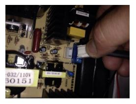
2. Remove screws (4) from the board, desolder the wires (4) from the thermoelectric module.
