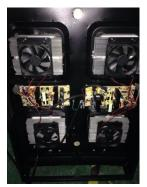
2. Remove the screws (2) on the Thermoelectric Module.
