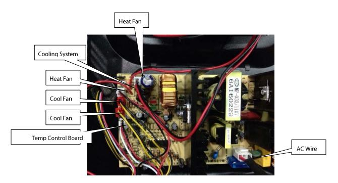
NOTE: All wiring connections need to be attached securely to the board.
