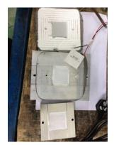
4. When replacing the thermoelectric node make sure it faces the correct direction and apply thermal grease evenly.
