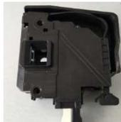
Step 3: Give a power pulse to the Lock between Pin 2 and Pin 3 again. The slipper should move back to its original place immediately. Otherwise, the lock is failing.
