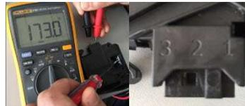
Step 2: Hold the Locker Slip Left as figure above. Give a power pulse to the Lock between Pin 2 and Pin 3. Then release the Slipper. It should take the place without any movement. Otherwise, the lock is failing.
