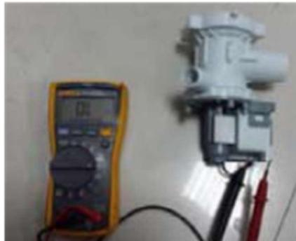
The resistance of coil should be in range from 30 to 40  $\Omega$ .
