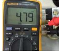
The resistance on coil should be between 3-5KΩ.
