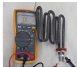
The resistance should be in range from 8 to  $15\Omega$ .
