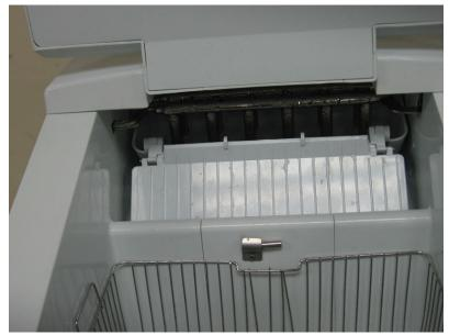
Here is a closer view of the hinge of an ice maker after installing a new ice shovel- fig. 7. Fig. 7:
