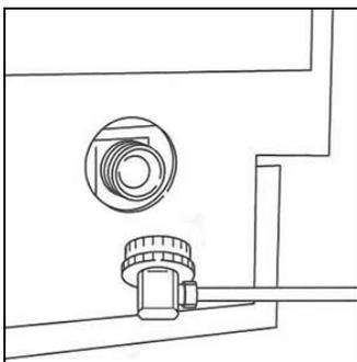
4. Lightly tighten the compression fitting around the water line with an adjustable wrench or similar tool.
