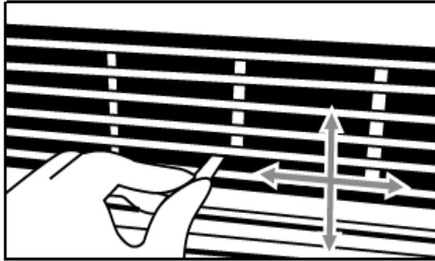
The 4-way air directional louvers allow you to direct the air flow Up, Down, Left, and Right throughout the room as needed. To adjust the air directional louvers side to side use the center handles as you move side to side.
