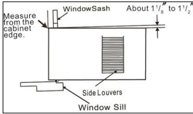
3. Check that the air conditioner cabinet is tilted back about 1 1/8" to 1 1/2", which should be about 3-4 degrees downward to the outside. After proper installation, condensation should not drain from the overflow drain hole during normal use, correct slope or otherwise.
