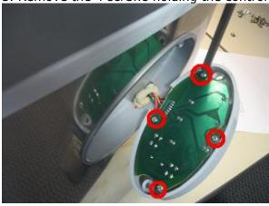
6. Remove the wiring connector from the control panel board.
