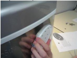
5. Remove the 4 screws holding the control panel board to the front cover.
