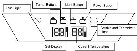
Use the up and down buttons to adjust the temperature. The temperature displayed can be in Fahrenheit or Celsius. This beverage cooler has a temperature range from 38°F to 50°F.
