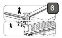
6. Carefully insert the door into the upper right corner hinge, then slide the door on top of the lower hinge and secure the door by installing the lower screws.
