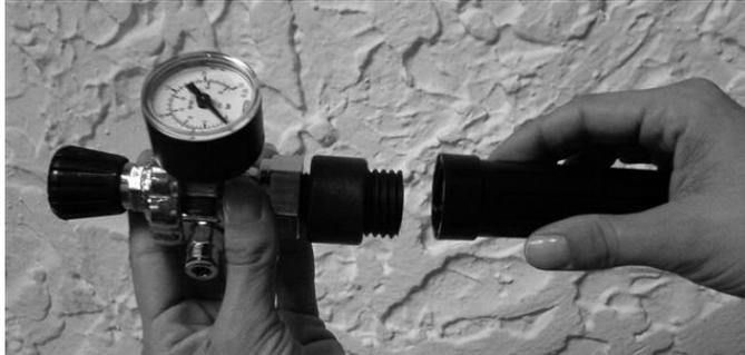
Note: once you screw this assembly together with a 16g CO<sub>2</sub> cartridge, do not unscrew it until the cartridge is empty- or all remaining CO<sub>2</sub> will rush out
