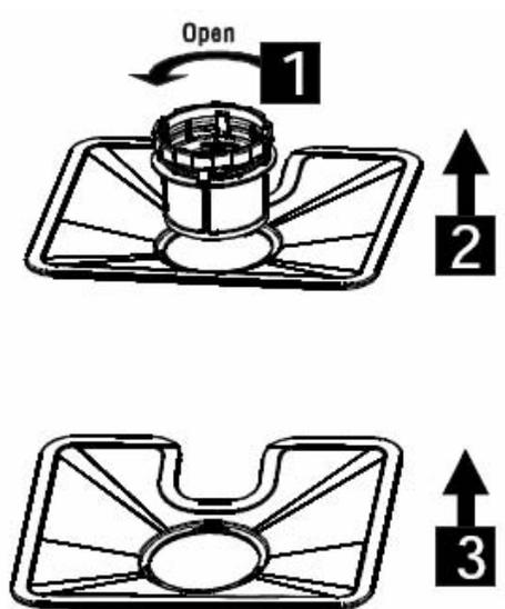
Step1: Rotate the fine filter counter-clockwise;
