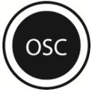
When the heater is in operation press the "Osc" to turn on the oscillation feature. The body of the unit will swing left and right automatically, at the same time the oscillation indicator light will illuminate. Press the "Osc" once more to turn oscillation off.
